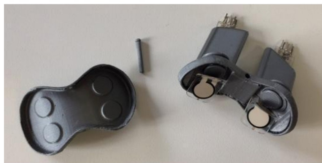
Figure 2. Interior of the instrument, showing the four sensors positioned in each quadrant
